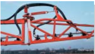
Breakaway wings automatically return to operating position
